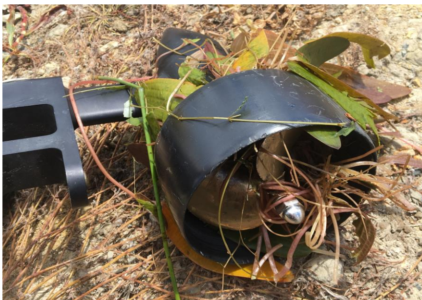
Photograph 2: One of the Q-boat propellers clogged with weed from a pond. The weed had to be removed before sampling could continue.
