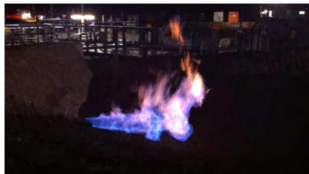
Figure 10. Syngas burning in the Huntly UCG flare pit shortly after ignition
