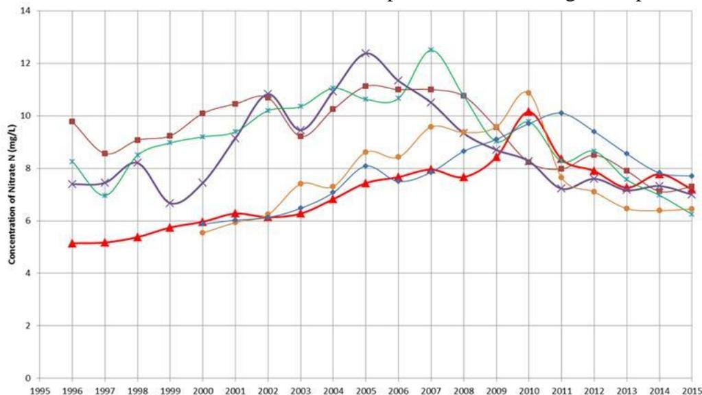
**Fig. 4.** Average annual nitrate-nitrogen concentrations in bores down-gradient of a dairy factory discharge
