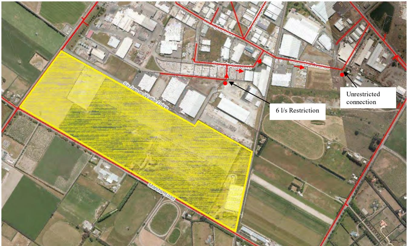
Figure 1: Site location with location of sewer restrictions
