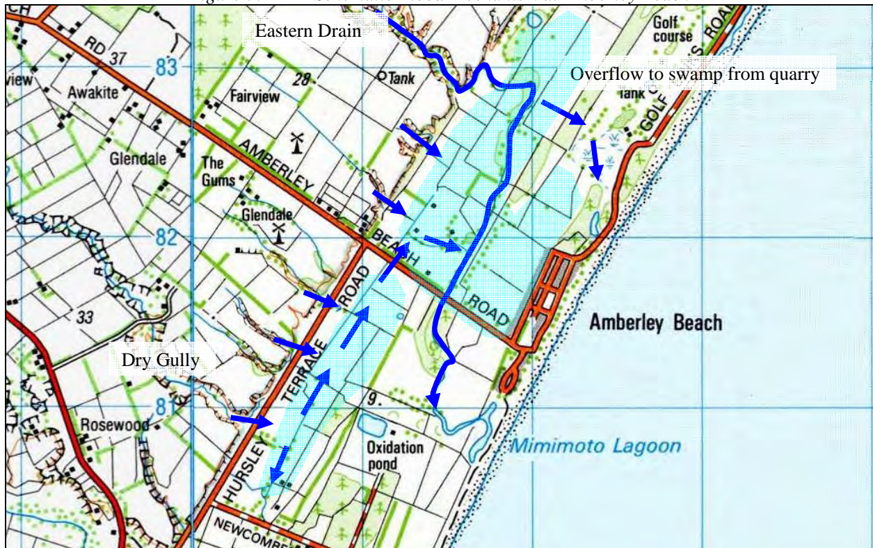
Figure 7: Schematic Flood Mechanism at Amberley Beach
