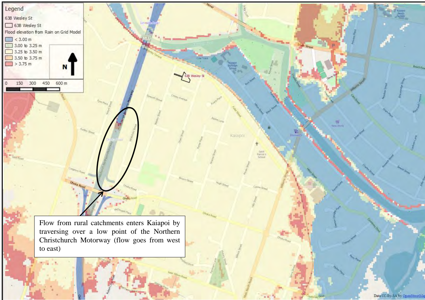
Figure 4: Flood elevation predicted by the WDC Rain on Grid Model for the 100 year ARI event
