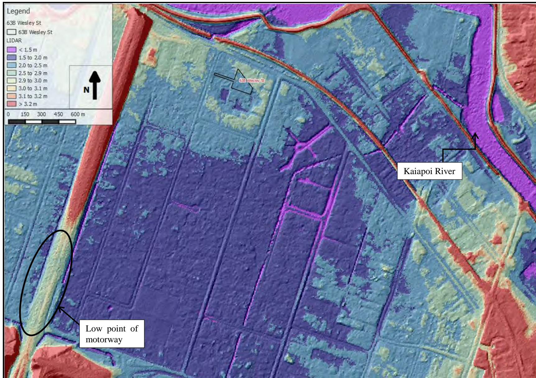
Figure 2: Post earthquake ground elevations derived from LIDAR data flow on 6 September 2010
