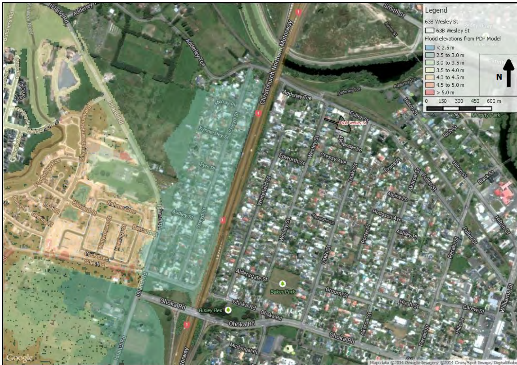
Figure 3: Flood elevation predicted by the PDP Model for the 50 year ARI event, note no overtopping of the motorway
