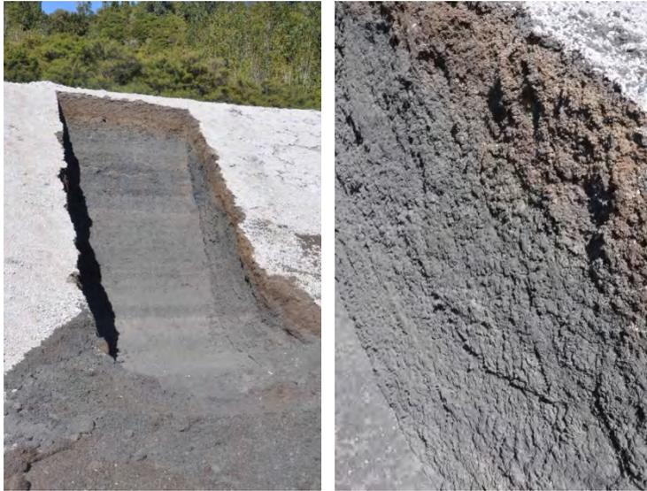
Figure 3. Compacted Primary Solids
